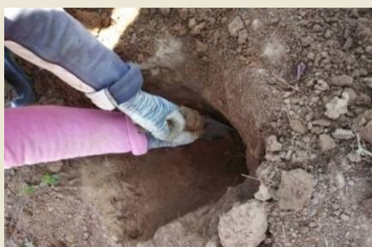
Fig 21. Digging of V shape pits and collect the soil slice
